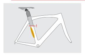
The maximum insert depth depends from the frame size:
